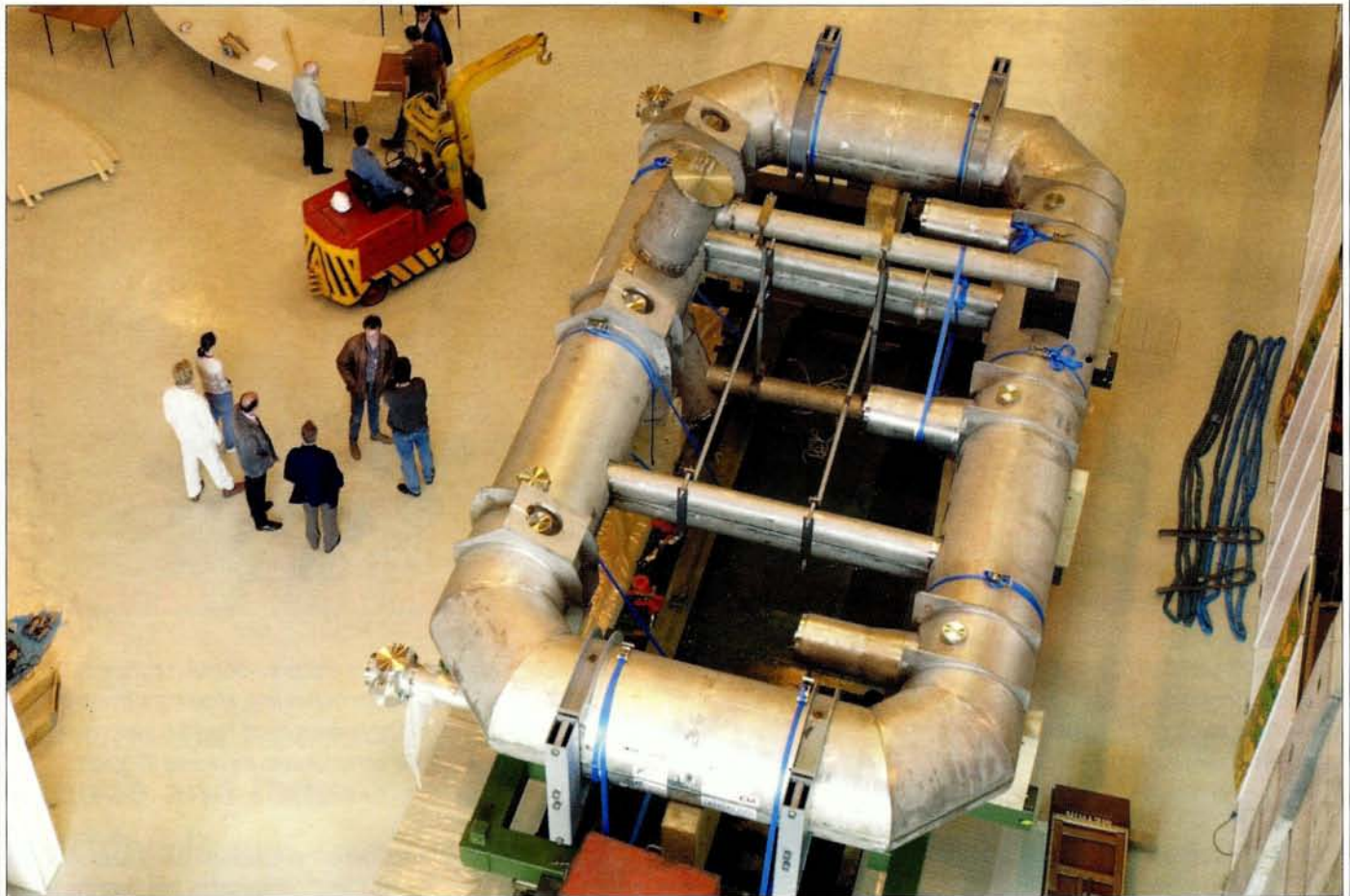
The ATLAS experiment's prototype B-0 toroid coil arrives at CERN from the CEA laboratory in Saclay on 6 October.
