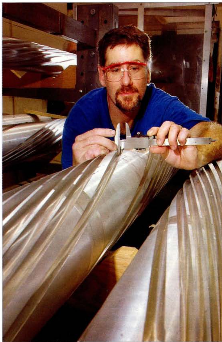
Brookhaven technician Chris Cleary puts together the "Siberian Snake" magnet string used to control spin-oriented (polarized) protons at the RHIC collider.
